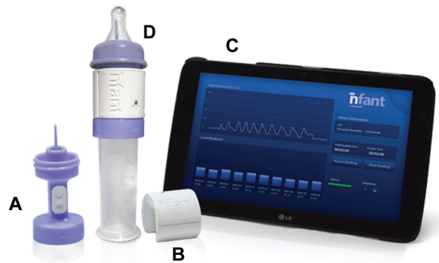
Figure 2. Components of the bottle-feeding system. (A) Bottle coupling with nipple cantilever. (B) Wireless sensor. (C) Recording tablet. (D) Fully assembled system.
